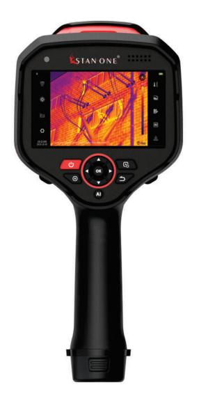
The STX 480 & STX 640 are power Inspection Thermal Imaging Cameras with "Interchangeable" lens options to allow configure as per application & distance requirement.
